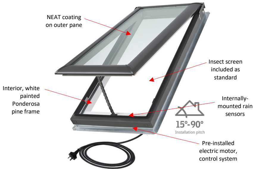
Figure 8. Velux Electric Skylight (VSE) - openable
