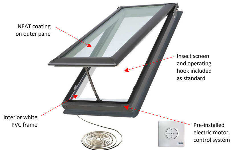
Figure 12. Velux Electric Skylight (VCE) – openable
